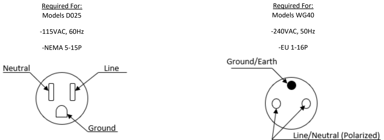
Fig. 1: Plug configurations
