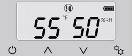
A digital display showing two temperature readings: 55°F and 50%RH. Above the 55°F reading is a small icon of a circle with an exclamation mark and the number 4. Below the display are four control buttons: a power button, an up arrow, a down arrow, and a settings gear icon. | <b>EL SISTEMA CONTINUA OPERANDO DURANTE ESTA ALARMA</b><br>Mala o nula transferencia de datos entre el sensor y el panel de control principal<br>"!4" permanecerá en la pantalla hasta que la comunicación sea restablecida. |
